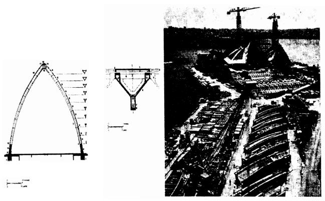
Fig. 4. Sydney Opera section and construction slide. Concrete prefabricated elements all different from each other had to be numbered. Courtesy of Phaidon (see bibliographical notes).
