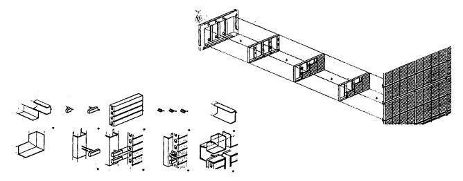
Fig. 7. IRCAM cladding system, showing how Renzo Piano rehearsed the construction/erection sequences. Courtesy by Phaidon. Peter Buchanam, Renzo Piano Building Workshop, Complete works, Vol. 1 Phaidon, 1993.
