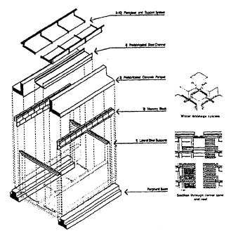
Fig. 3. Herman Hertzberger Central Beheer Office Building. Deconstructed detail of roof drainage and skylight. Drawing by Hans Houser.
